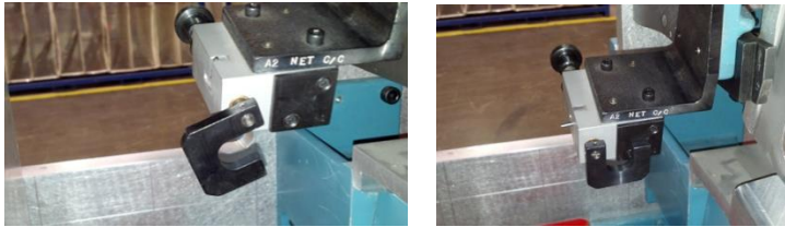
Hook/swing in clamp to clip attachment
